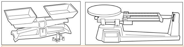
A pan balance (left) compares the masses of different objects. The pan holding the more massive object sinks, while the pan holding the less massive object rises. A triple-beam balance (right) is used to measure the mass of an object. It typically provides more precise measurements than a pan balance.
